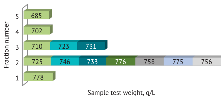
Figure 3. Results of the investigation of test weight samples for each fraction under the operating mode with the grain feed lever set to “1” and the fan airflow lever set to “3”
